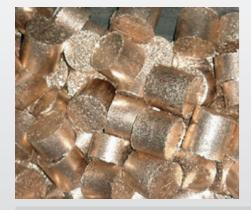
CHIP RECYCLING OPTIMISED THROUGH **BRIQUETTING IN CHANNEL FURNACE**
