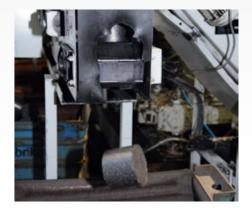
Briquetting system: RUF 30/3700/100 (adapted model)
